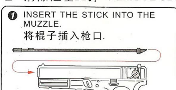
PREMOVE THE CLOGGED BULLETS. 清除阻塞的BB弹.
